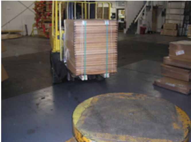
Rail parts were stored on 2 x 4 runners which resulted in significant bowing and waste.
